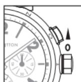
To restart the movement, manual winding is recommended. In position 0: wind by turning the crown clockwise 20 to 30 times. The movement will then wind up automatically each time the wrist moves.
